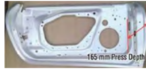
Fig 6: Hot Form Quench Process to achieve complex formed shape and optimised metallurgical properties with zero spring back in most cases. Condition of the part after age hardening... see illustration graph below. And distortion/spring back b & c.
