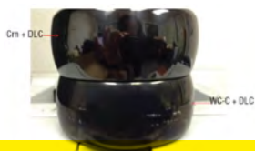
Fig 7. forming tools DLC family composite Top section tool, Chromium Nitride (CrN) + DLC, Bottom section tool, Tungsten Carbon
