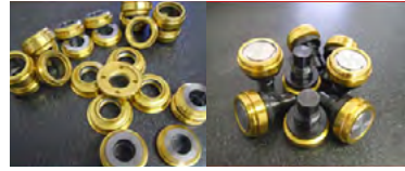
Seaming Rolls Chemical Vapour Deposition coated with 8µ thick layers of TiC/TiCN/TiN
