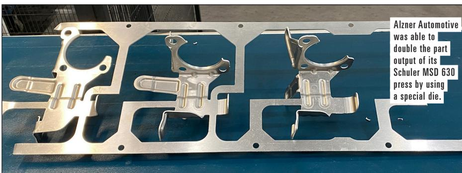
Alzner Automotive was able to double the part output of its Schuler MSD 630 press by using a special die.
