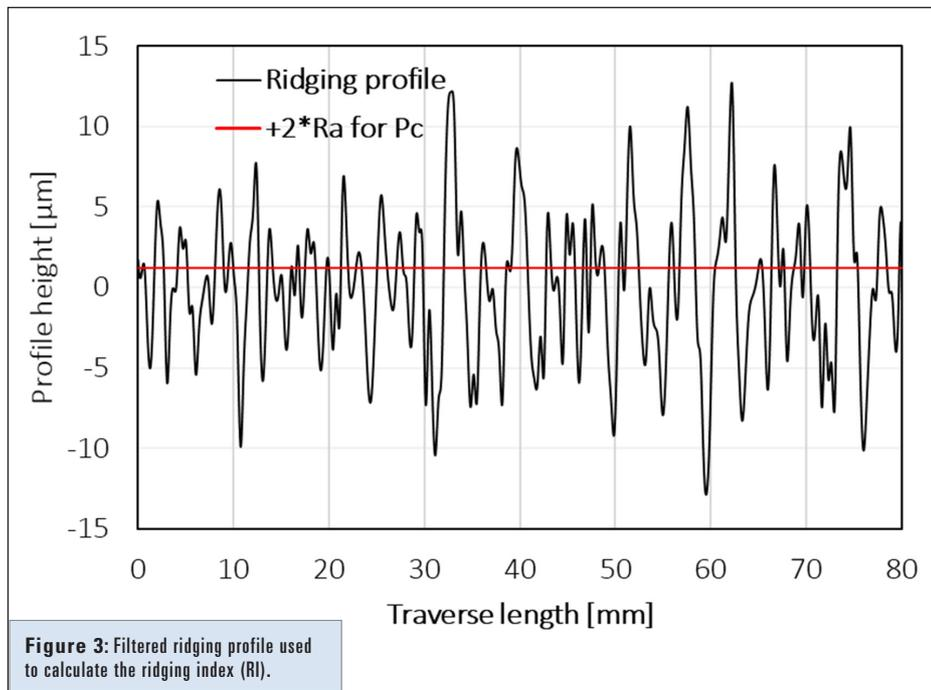
**Figure 3:** Filtered ridging profile used to calculate the ridging index (RI).
