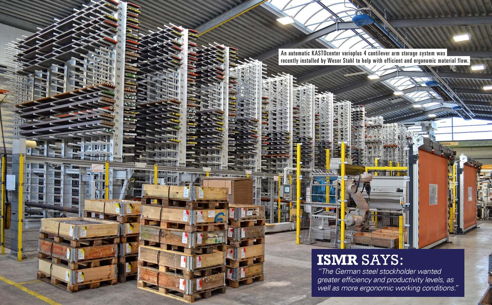
An automatic KASTOcenter varioplus 4 cantilever arm storage system was recently installed by Weser Stahl to help with efficient and ergonomic material flow.
