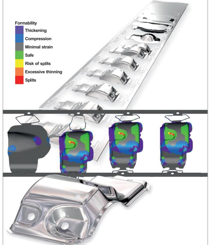
Logopress ProgSim enables progressive die designers working in SOLIDWORKS to efficiently simulate, modify, and validate their strip layouts. The software allows them to gain deep insight into the forming process and take corrective measures on the computer screen to prevent costly prototyping and/or trial and error in the tryout press.
