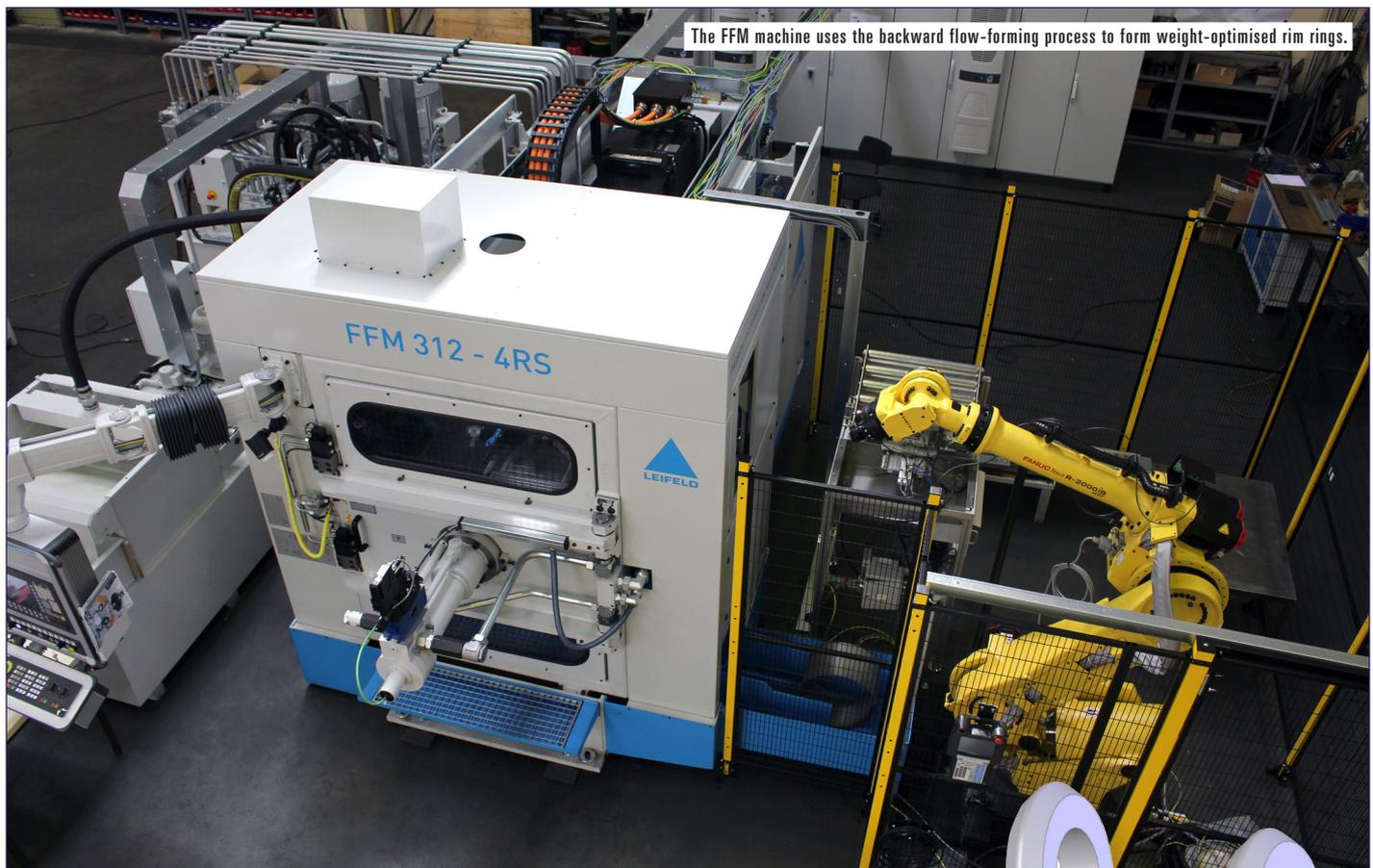
The FFM machine uses the backward flow-forming process to form weight-optimised rim rings.
