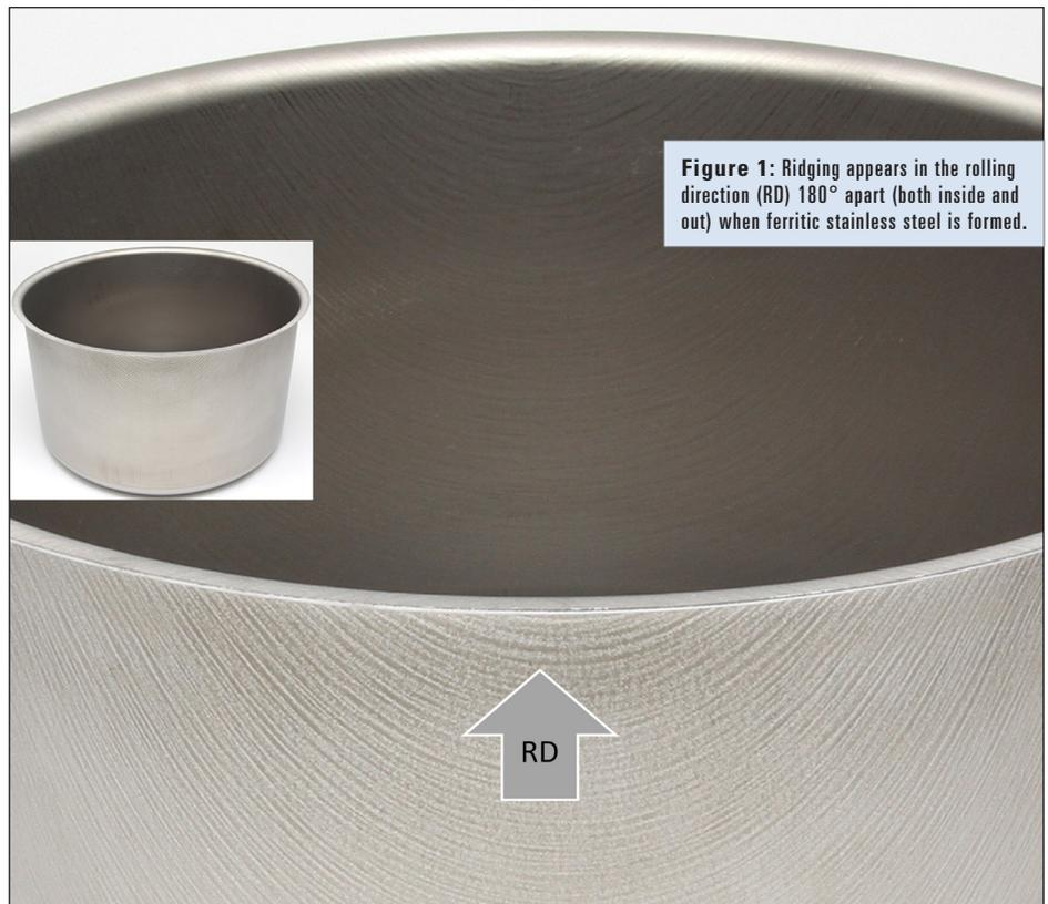
**Figure 1:** Ridging appears in the rolling direction (RD) 180° apart (both inside and out) when ferritic stainless steel is formed.
