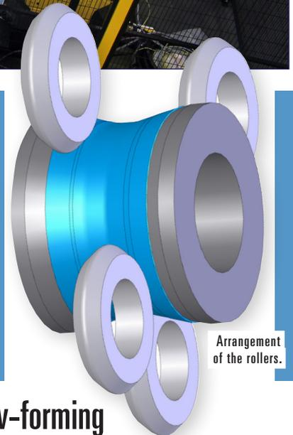
**Less weight means fewer CO<sub>2</sub> emissions for cars and trucks. Flow-forming enables the chipless production of weight-optimised wheels, without loss of payload.**
