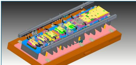
affect the transfer tooling. In some transfers automated by Misati, a reduction of just 100mm in the distance between dies (from 600 to 500mm) has generated an increase of more than 20% in the number of strokes per minute.
