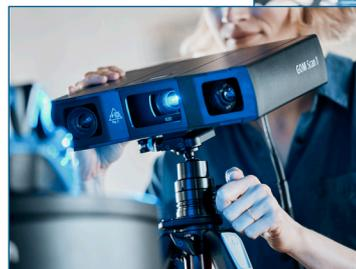
sensor software continuously monitors the calibration status, transformation accuracy, environmental changes and part movements. GOM Scan 1, with GOM Inspect, delivers accurate and comprehensive measurement results making 3D part inspection effortless. With the software, users can easily import and align CAD and mesh files, create surface comparisons or dimensional inspections and generate reports," added GOM.
