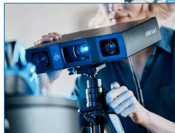
sensor software continuously monitors the calibration status, transformation accuracy, environmental changes and part movements. GOM Scan 1, with GOM Inspect, delivers accurate and comprehensive measurement results making 3D part inspection effortless. With the software, users can easily import and align CAD and mesh files, create surface comparisons or dimensional inspections and generate reports," added GOM.
