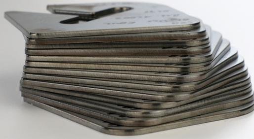
Metallic blank cut surfaces with the HiFinox technology for plasma cutting of stainless steel and aluminium (© Photo: Kjellberg Finsterwalde).
