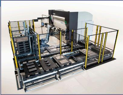
LVD's Ulti-Form robotised bending cell handles parts from 50 x 100mm up to 1200 x 800mm (\*weighing up to 25kg).
