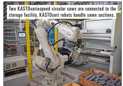
Two KASTOvariospeed circular saws are connected to the storage facility. KASTOsort robots handle sawn sections.
