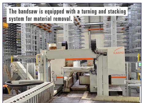
The bandsaw is equipped with a turning and stacking system for material removal.
