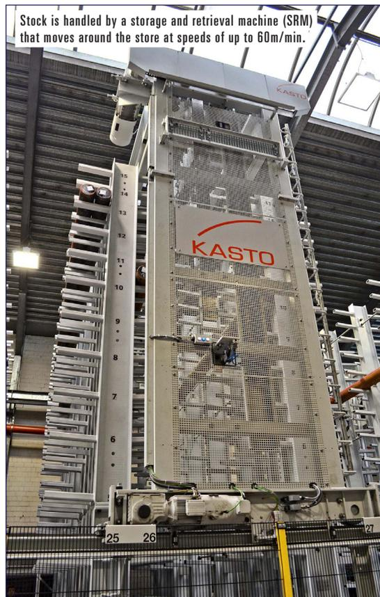
Stock is handled by a storage and retrieval machine (SRM) that moves around the store at speeds of up to 60m/min.
