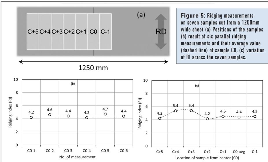
The RIs of all seven specimens are shown in Figure 5(c). Four of them are similar to C0, the centre sample. The two samples furthest from the centre of the sheet showed RI values of about one unit higher. This could possibly indicate a locally different texture in the FSS sheet.
