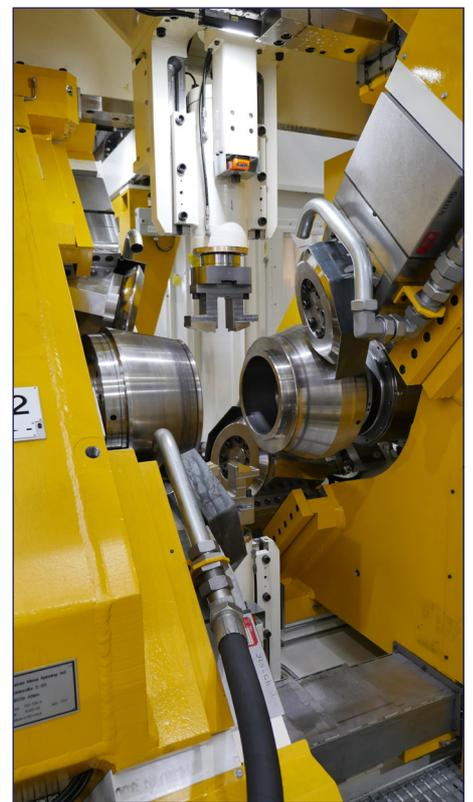
Above: A view of the working area of the Leifeld RSC Series with four flow-forming rollers.
