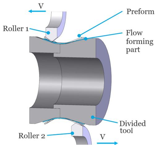
Above: Bi-conical forward flow-forming by Leifeld's RSC and RC series machine process.
