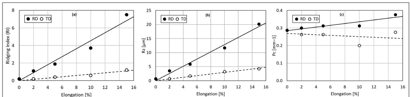
**Figure 4:** The influence of strain and straining direction on the ridging index (RI).
