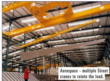
Aerospace - multiple Street cranes to rotate the load.
