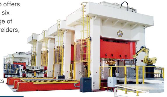
Above: An HD-2500 press tandem line, with robotic arm feeder, from DEES Hydraulic.
