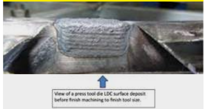
Fig 2 Back of die wall showing weld deposit
