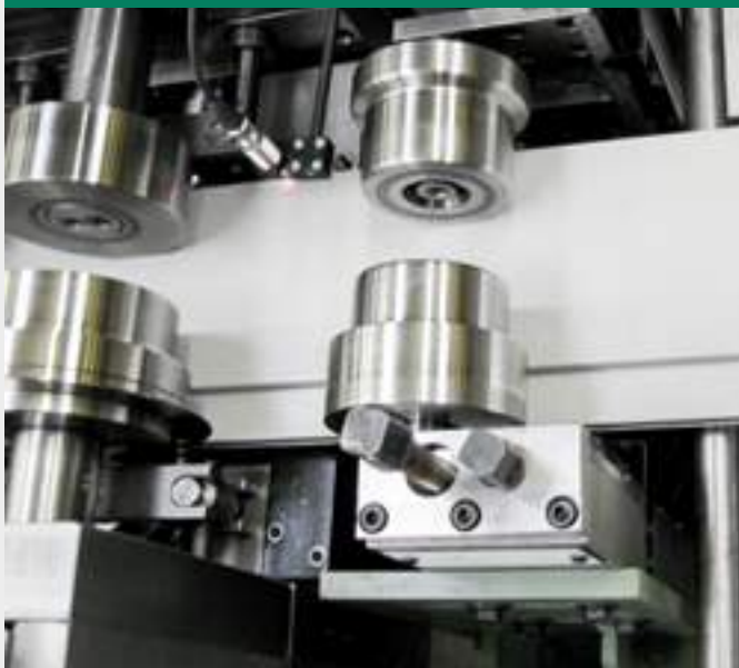
Duplex roll former forming from flat blanks forming face panels
