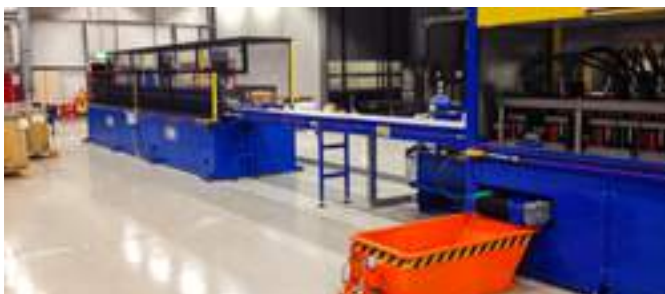
Conventional roll forming line with pre punching and pre cut to length
