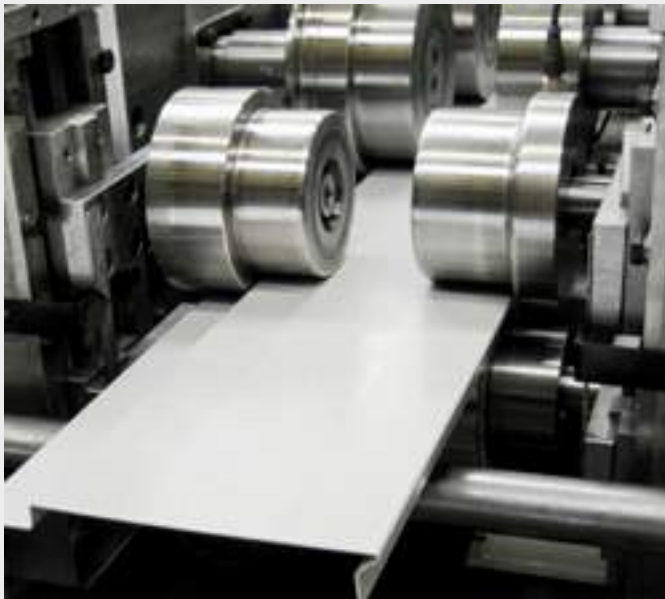
Duplex roll former forming from flat blanks forming face panels
