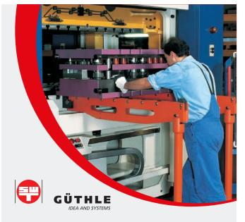
Systems designed for the world of hydraulic quick clamping and for professional quick die change, whether manual or automatic.
