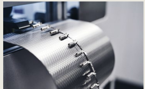
Step 3 The result is complex components which can be produced incredibly efficiently, at stroke rates of up to 600.
