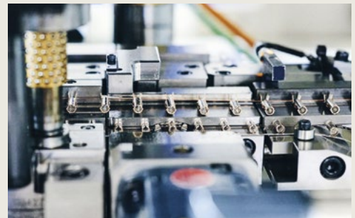
Step 2 The plug contacts have an internal spring added directly in the stamping press.
