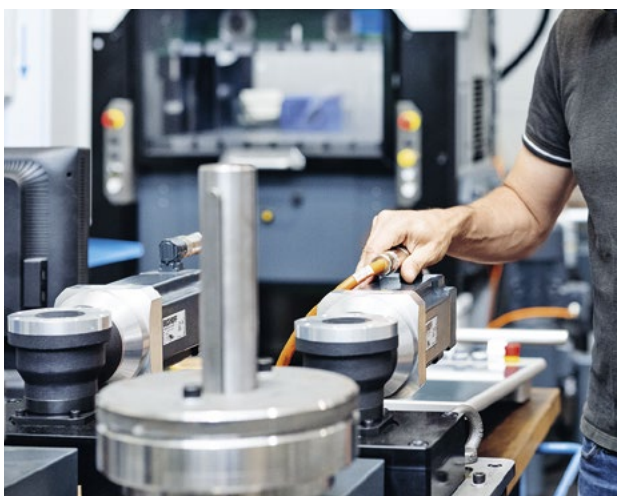
Freely programmable rotating stations make it possible to produce lamination stacks in various shapes.
