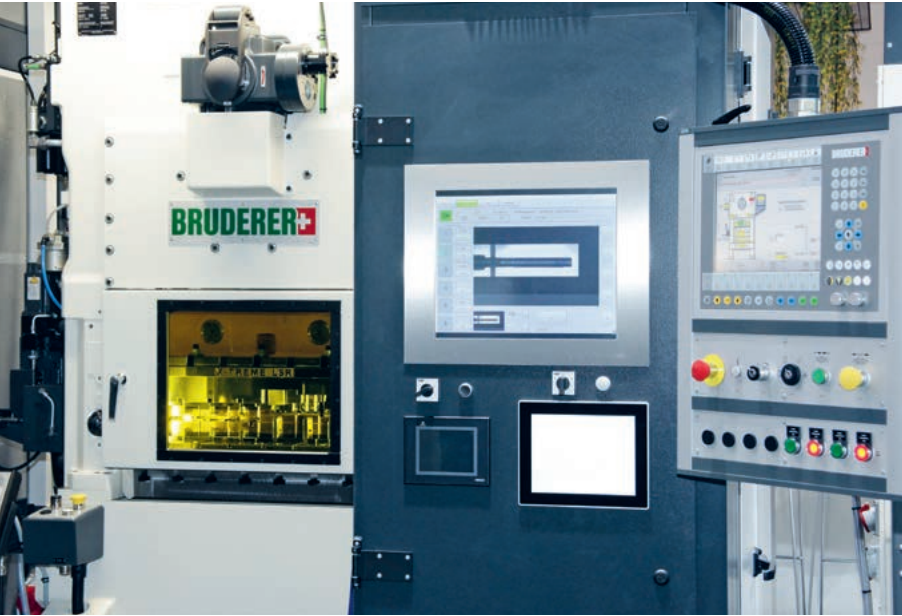
At Blechexpo, Stepper presented integral sensor-based weld monitoring in a BRUDERER BSTA-200/70 stamping press.
